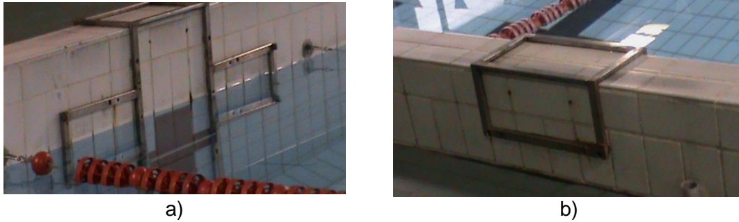
Figure 4. Underwater structure used by de Jesus et al. (2011; 2013) to fix one force plate, frontal (a) and posterior view (b).
