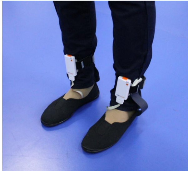
Figure 1. WalkinSense® and Pedar® attached on one of the participants during data collection.
