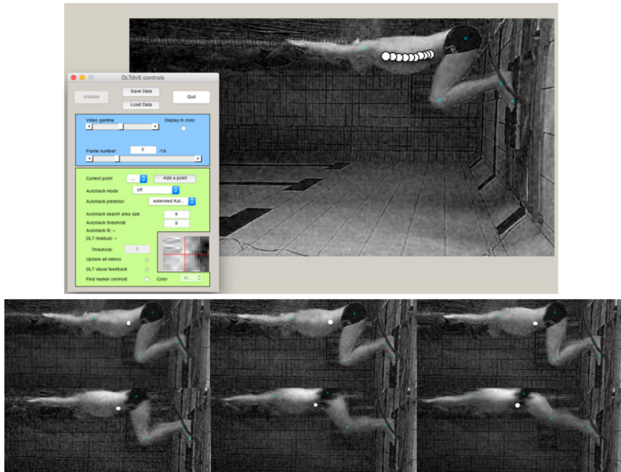
Fig. 3. Digitization software interface (upper panel) with position of anatomical landmarks in cyan dots. The accuracy of the digitization process is exemplified for the toes (red dot) on the left window. White dots symbolize CM trajectory throughout the push-off. Body positions, anatomical landmarks digitization and resulting CM positions during the maximal push-off are presented (lower panel). (For interpretation of the references to colour in this figure legend, the reader is referred to the web version of this article.)
